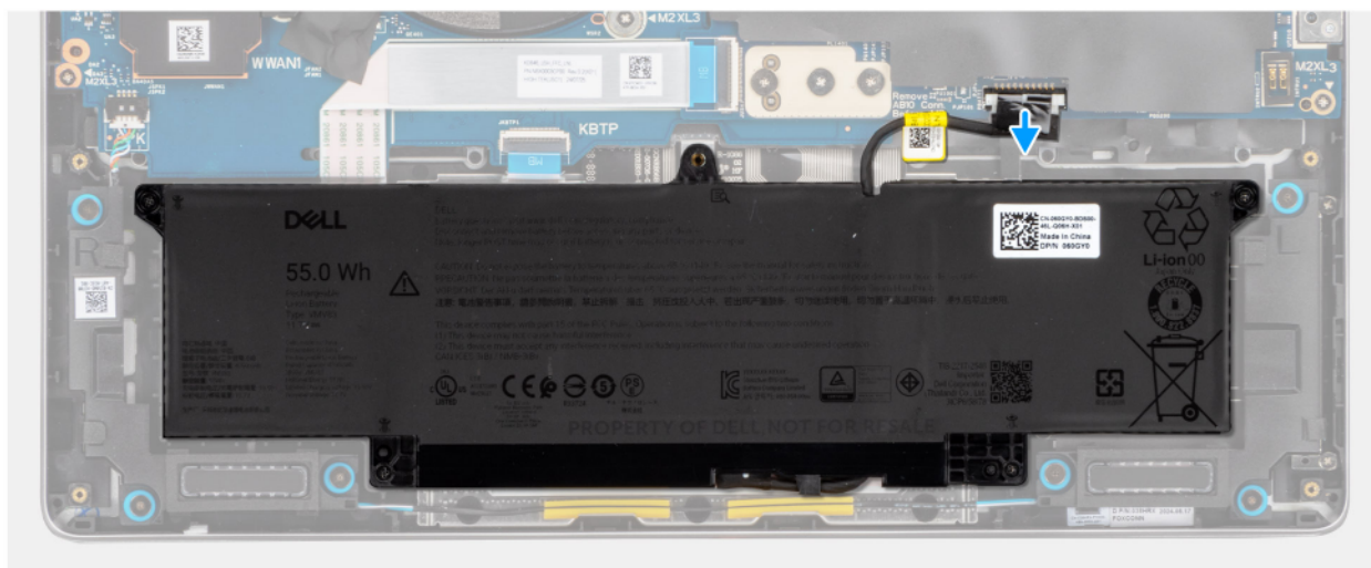
Figure 21. Disconnecting the battery cable
