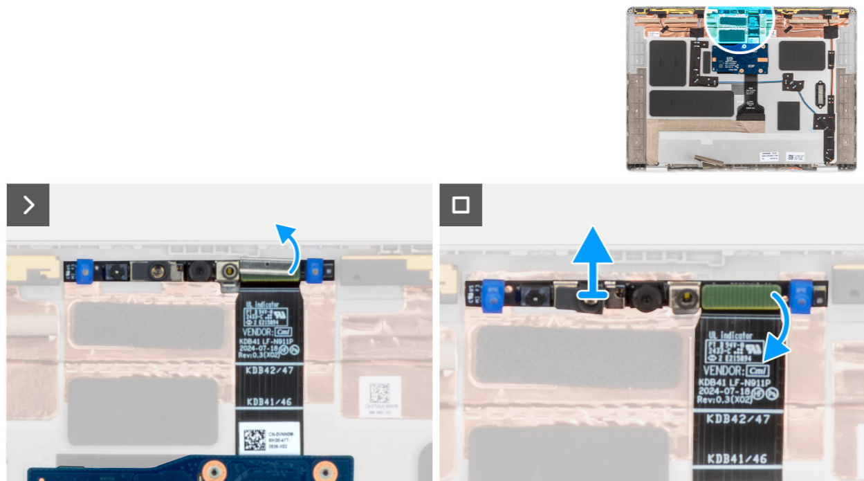
Figure 56. Removing the MIPI camera
