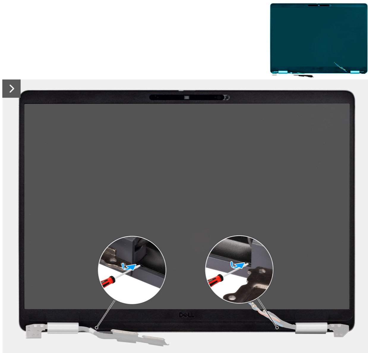
Figure 43. Prying the plastic bezel
