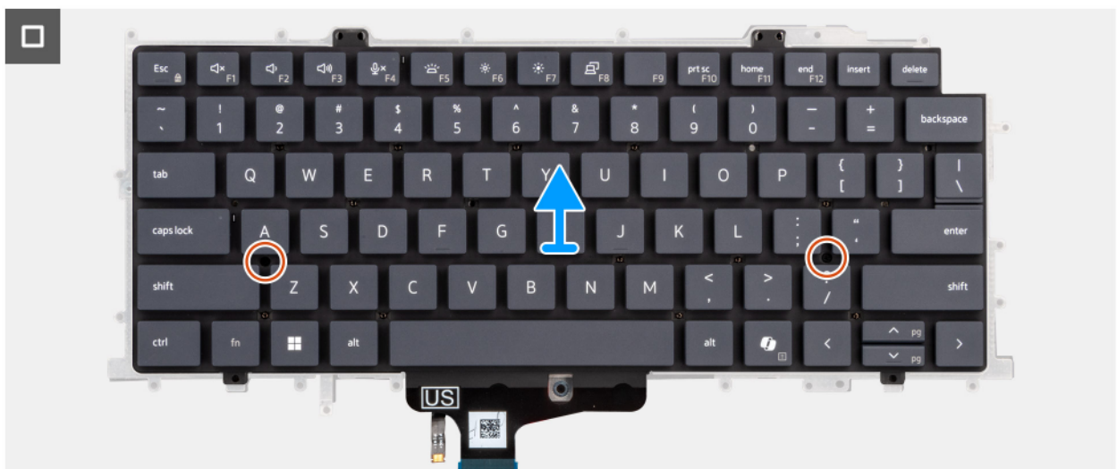
Figure 80. Removing the keyboard
