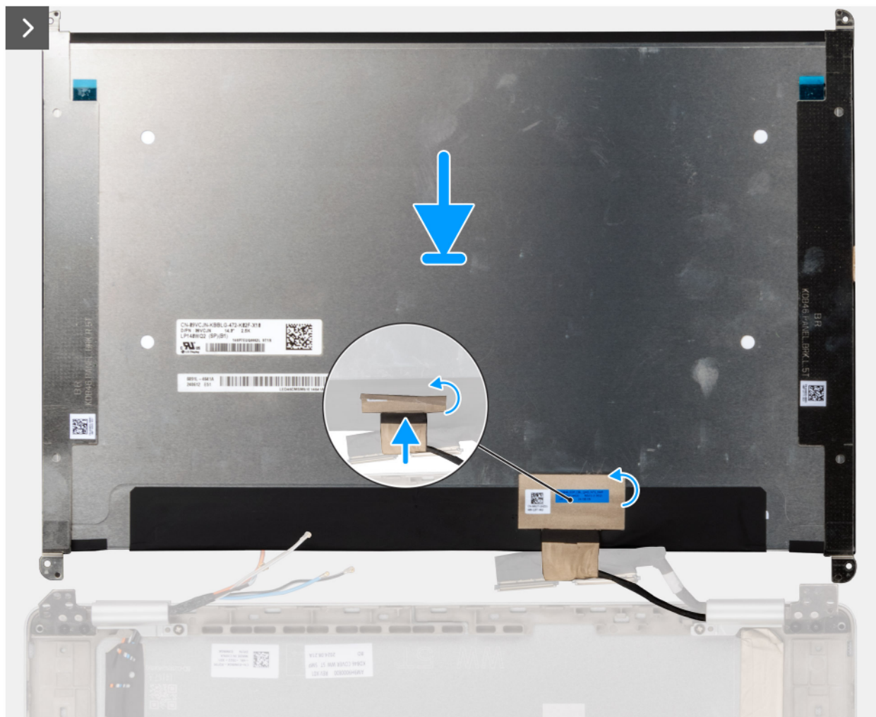
Figure 52. Installing the display cable
