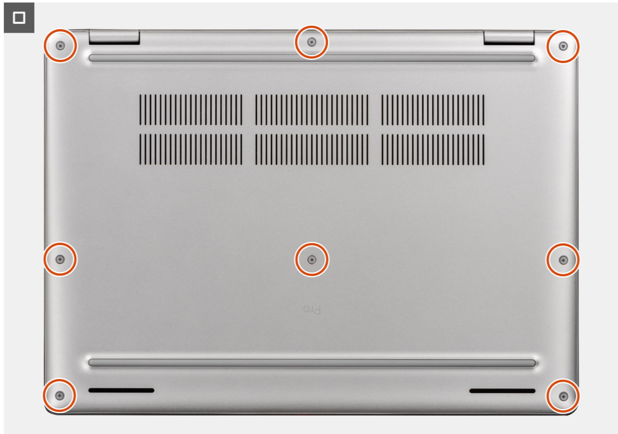
Figure 23. Installing the base cover
