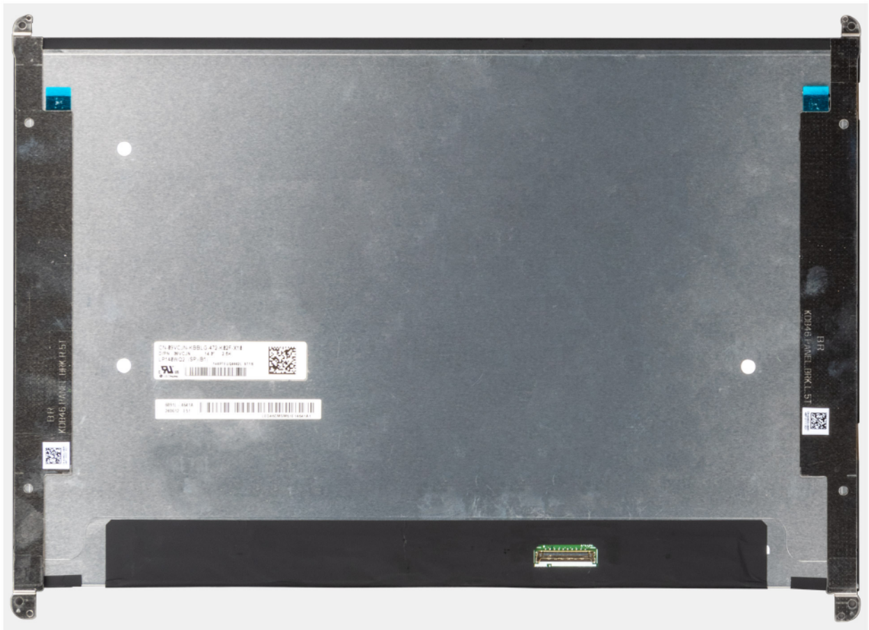
Figure 51. Display panel with brackets
