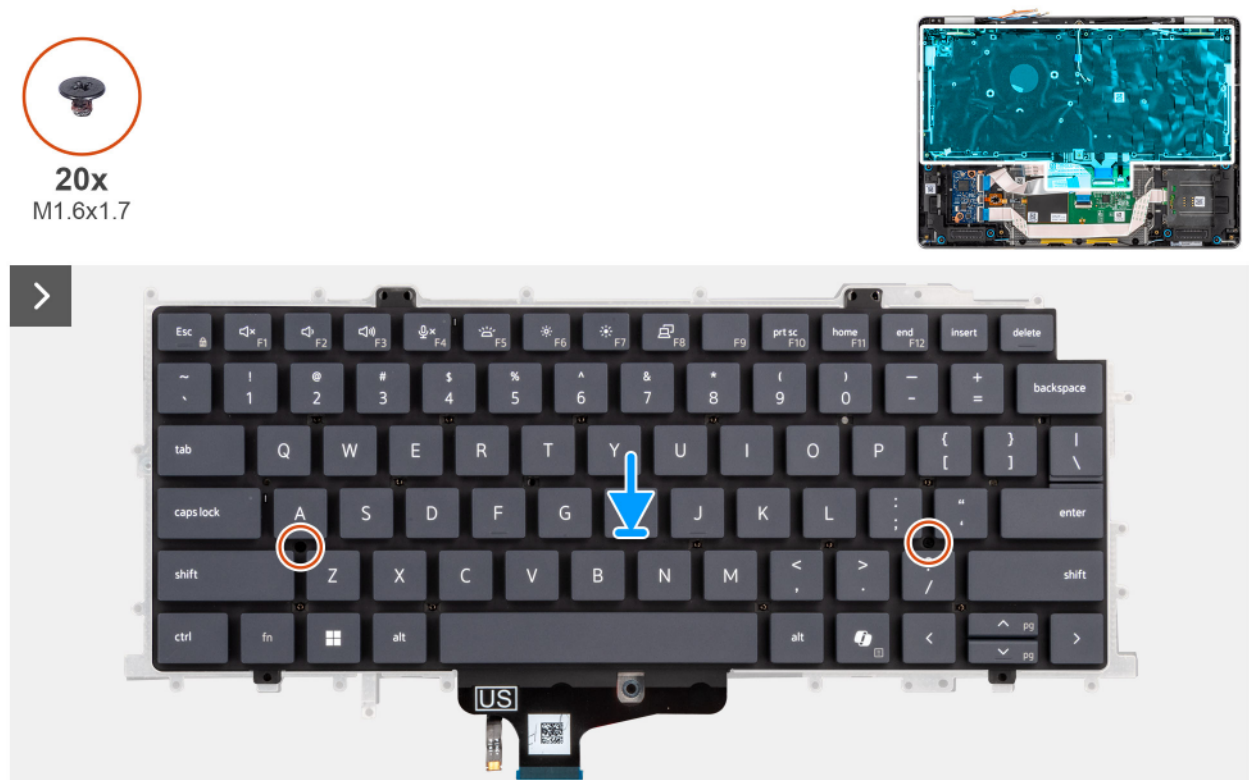
Figure 81. Installing the keyboard
