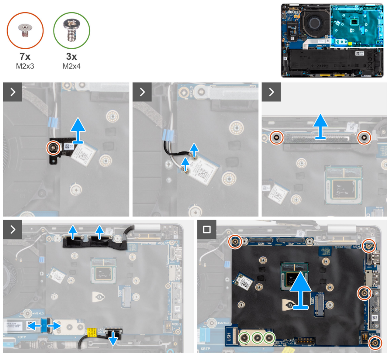
Figure 70. Removing the system board
